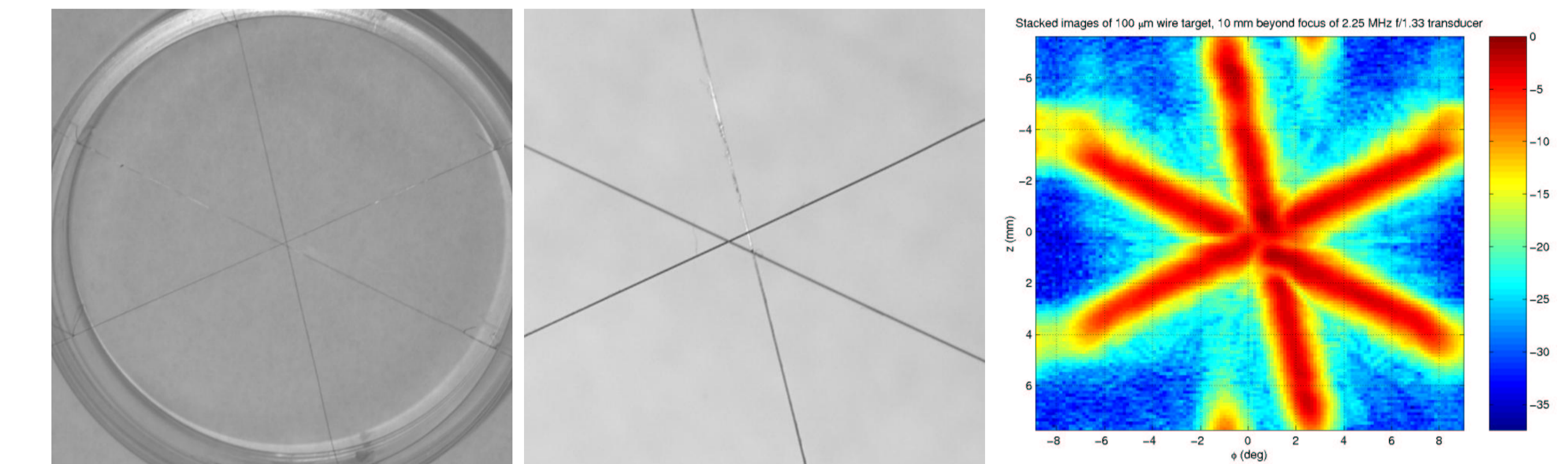
Left and center: 100-micron wire target and holder. Right: Reconstructed images of the target, stacked over depth, log scale.
